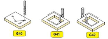
The diagrams show a milling tool cutting a square groove. In the G40 diagram, the tool is centered in the groove. In the G41 diagram, the tool is shifted to the left side of the groove. In the G42 diagram, the tool is shifted to the right side of the groove.
