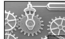
MicroElectroMechanical (MEMS) devices 10 -100 μm wide
