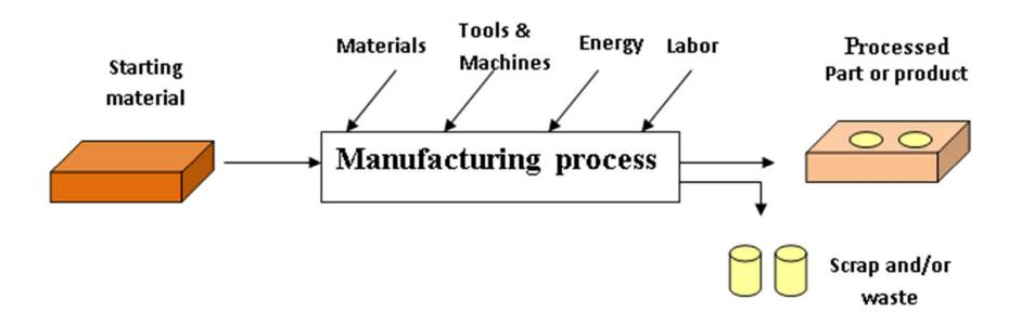
Figure 1.1- Manufacturing as a technical process
