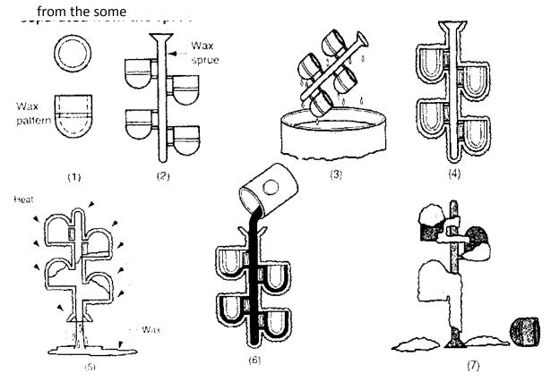
Figurel.19 Steps of investment casting casting process
