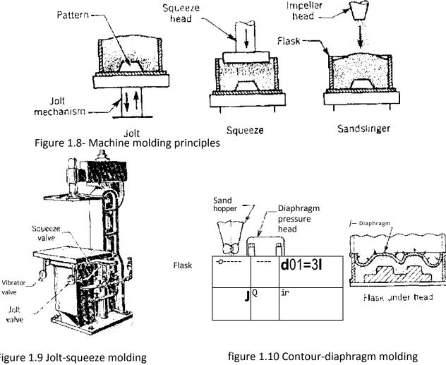
Figure 1.9 Jolt-squeeze molding machine
