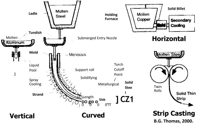
Figure 1. Various continuous casting processes
