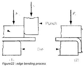
Bending of a metal sheet or plate into particular
