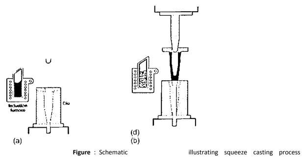
operations, (a) Melt charge, preheat, and lubricate tooling, (b) Transfer melts into die cavity, (c) Close tooling, solidify melt under pressure, (d) Eject casting, clean dies, charge melt stock.
