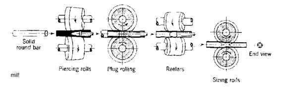
*Figure 7: Principal steps in the manufacture of seamless tubing.*
