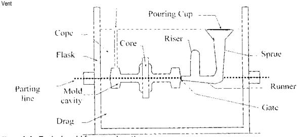
Figure 1.4 - Typical mold for a sand casting
