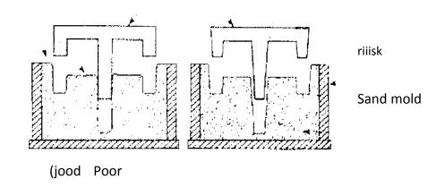
Figure 1.6 - Taper consideration in sand casting
