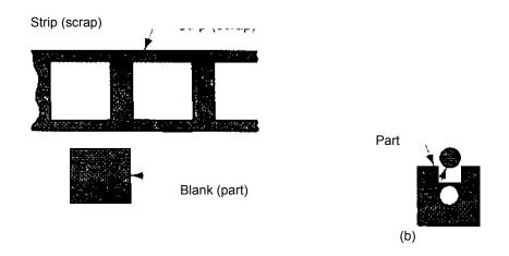
Figure 26: (a) Blanking and (b) Punching
