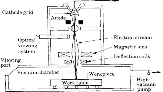
Figure : An electron beam welding process
